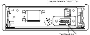
26 PIN FEMALE CONNECTOR: when there is some dirt on the connector, please wipe it away from the connector.
